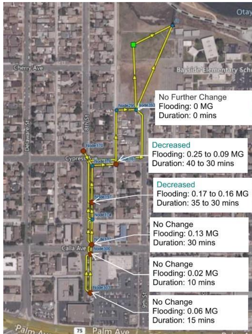
Figure 8 Implementing a detention basin provides isolated flood reduction benefit at Cypress Avenue, but not in areas south, due to the limited conveyance capacity in the stormdrain system between Cypress Avenue and Palm Avenue.
