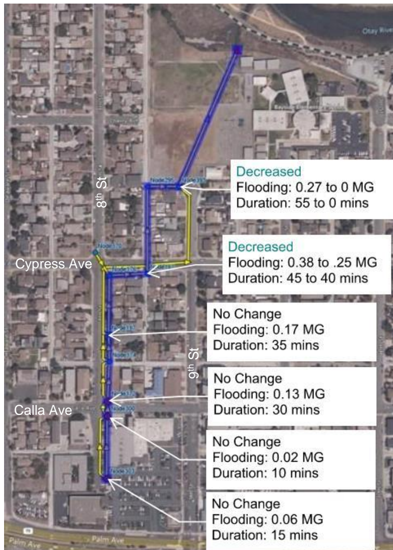
Figure 6 Implementation of a tide gate and open channel decreases flood volume and duration north of Cypress Avenue, but does not change flooding further south in the system.
