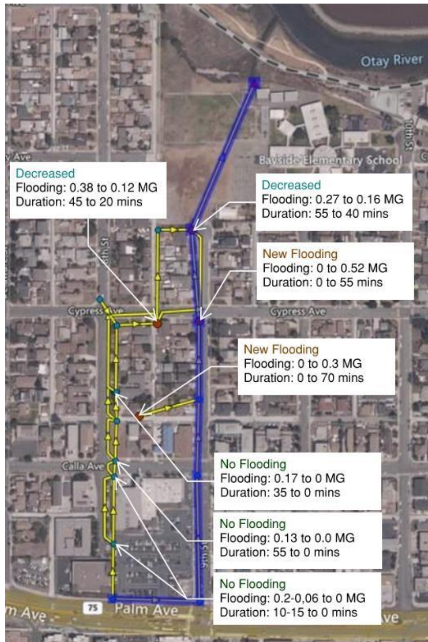
Figure 9 The historic high tide and 10-year storm event, flood reduction and increased flooding varies with implementation of the proposed NV5 parallel system.
