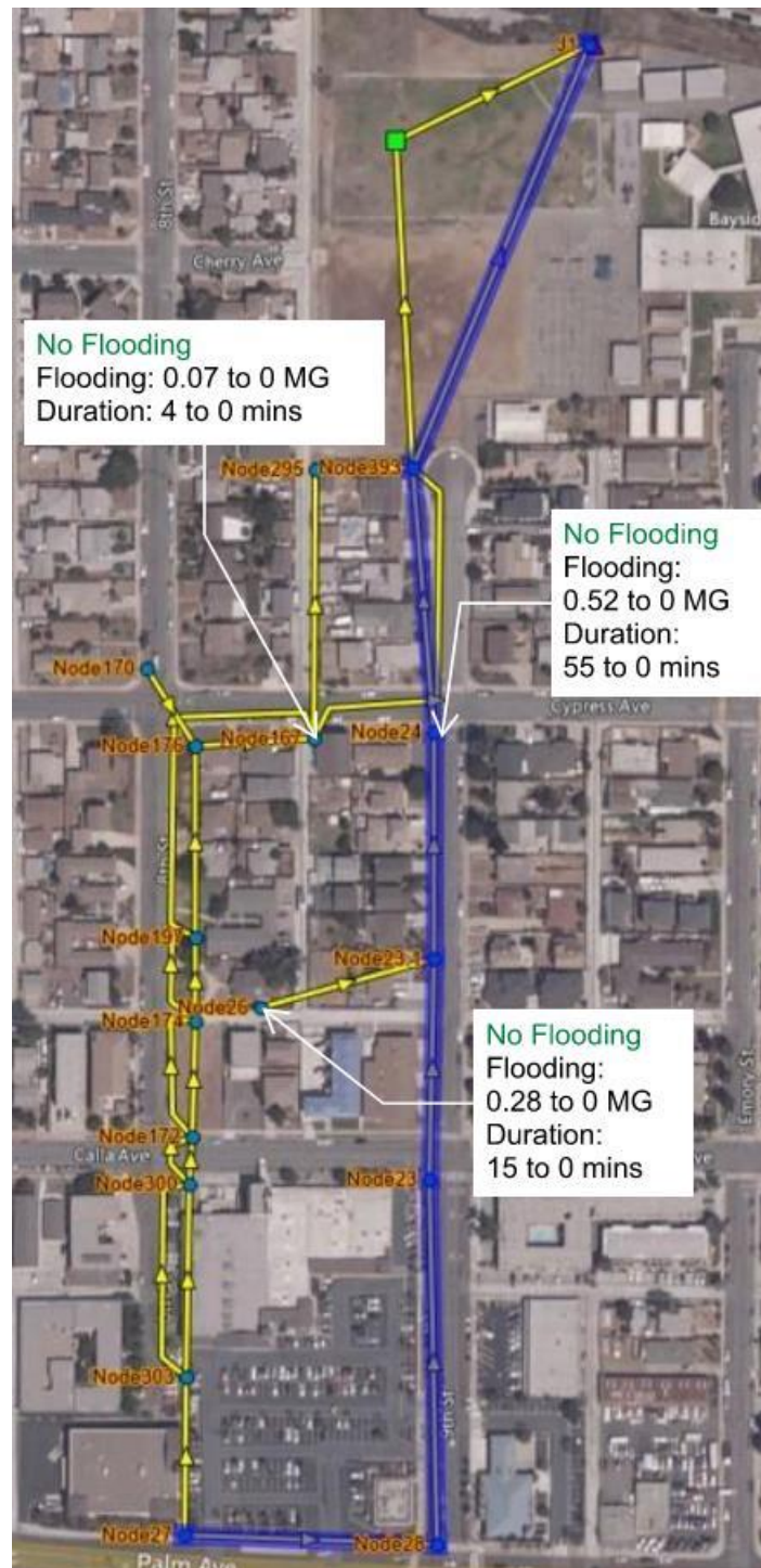
Figure 11 The tide gate, open channel and detention basin provide conveyance and storage in the system between the outfall and Cypress Avenue, while the parallel system increases the capacity of the overall system and reduces flows along the existing alignment.
